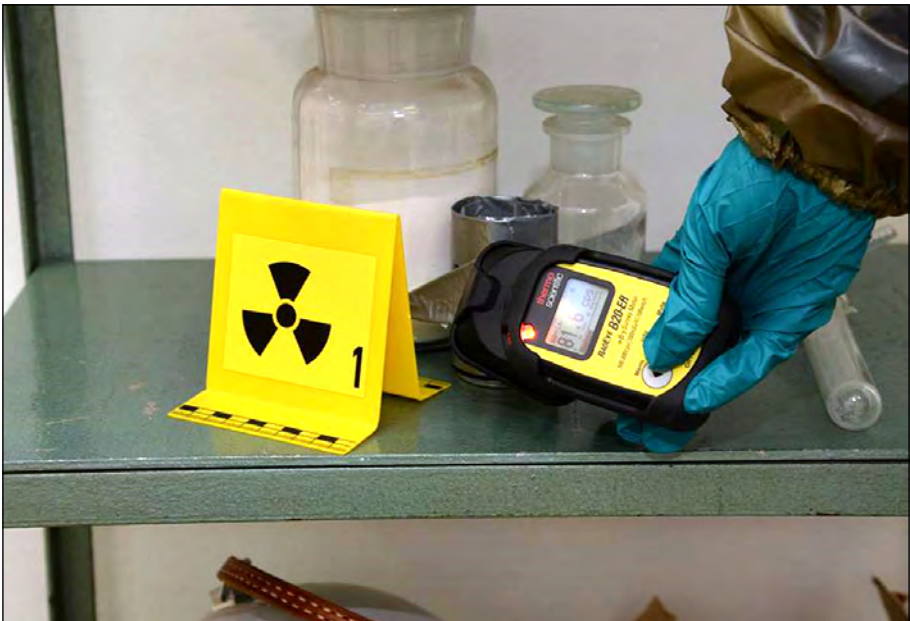
Fig. 6: Detection and marking of radioactive material
