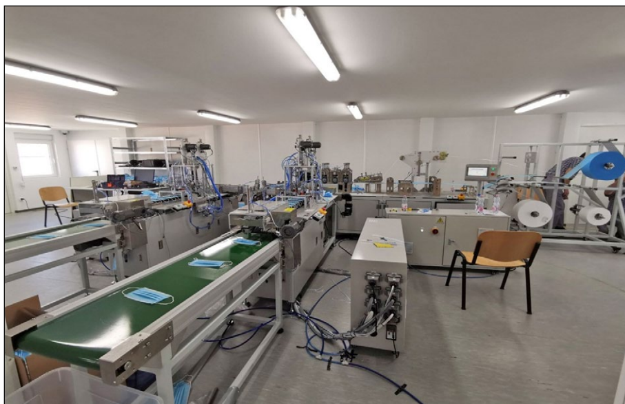
Picture 3: Disposable medical face mask production line
