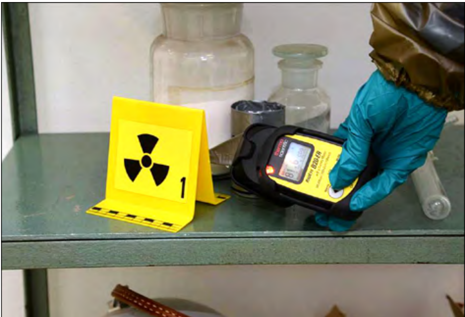
Fig. 6: Detection and marking of radioactive material
